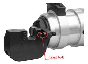
(2) Insert the steel bar fully into the U-shaped groove. Make sure that the rebar is fixed on the end plane of the bolt as shown in the diagure.
