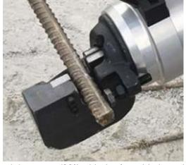
(3) Keep the steel bar at the right corner (90°) with the front blade and unscrew the
